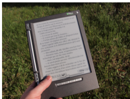
An e-reader with an EPD display
