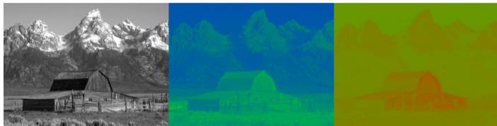
Decomposition in Y, U and V channels
