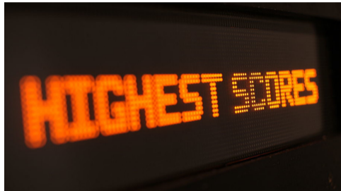
A monochrome dot-matrix display
