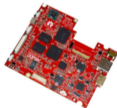
Olimex Open hardware ARM laptop main board
