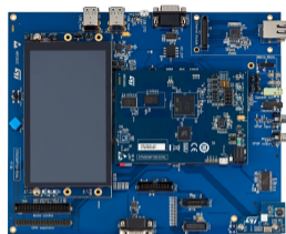
STM32MP157C-EV1 evaluation board
